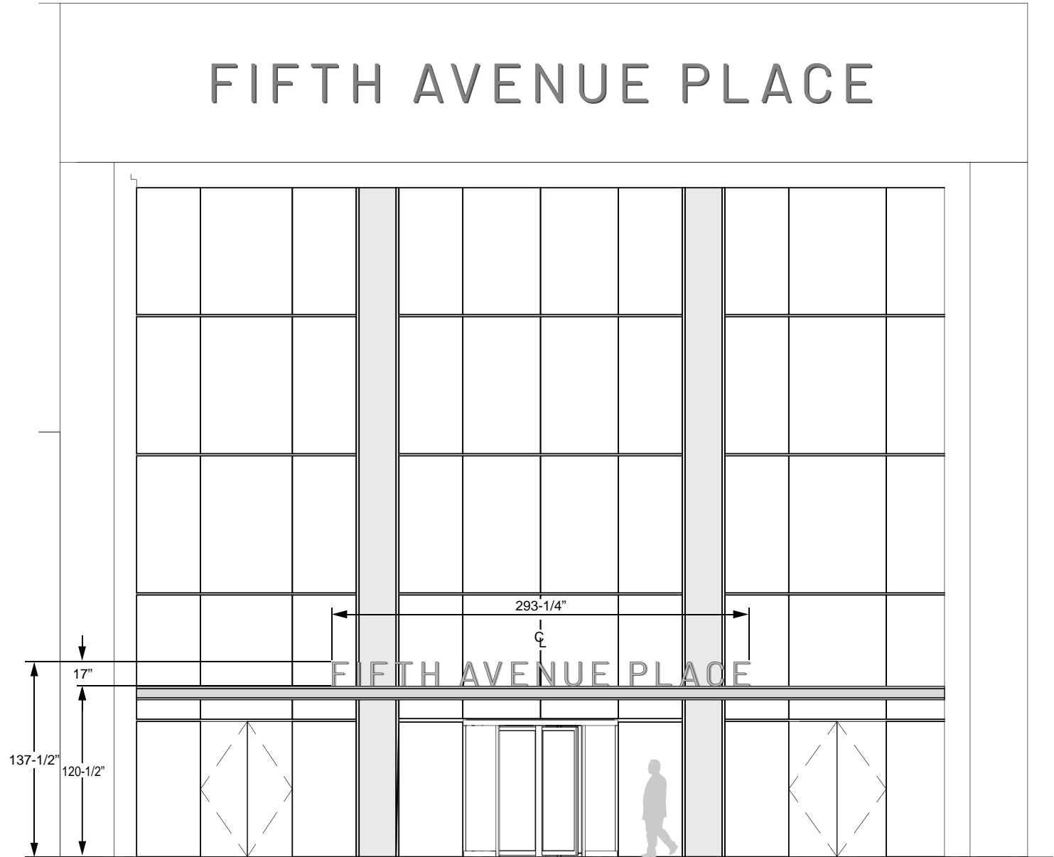
1 8 PROPOSED LIBERTY AVENUE CANOPY ELEVATION SCALE : 1/8" = 1'- 0"
