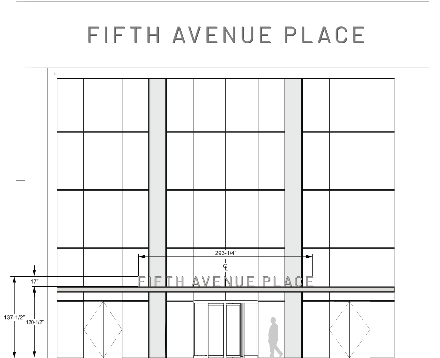
1 8 PROPOSED LIBERTY AVENUE CANOPY ELEVATION SCALE : 1/8" = 1'- 0"
